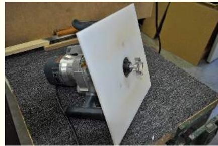
**Slab Cutting Jig & Plunge Router With UHMW Plate And Spoilboard Router Bit**
