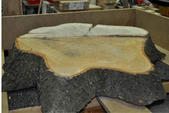
**Slab After First Pass With Router**
