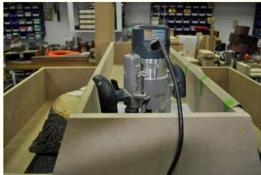
**Slab Flattening Jig In Operation**
